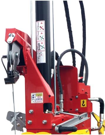
..... ● TREUIL HYDRAULIQUE AVEC REGLAGE VITESSE
